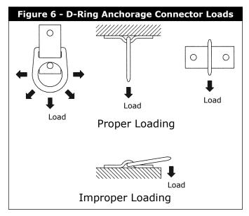
direction(s) of intended use to 3,600 lbs (16 kN). Protect finished welds from corrosion with paint or other finish. Do not electroplate the D-ring. Installations should be verified by a qualified person for strength by calculation in the intended direction(s) of intended use.
